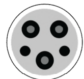
Side view (Left) and Charging Interface (Right) of a J1772 charge port used with Level 1 and Level 2 charging equipment
